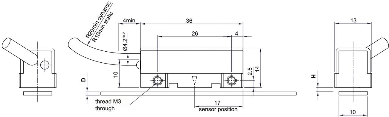
**NOTE:** Ensure recommended M3 readhead fixing screws are tightened to 0.5 Nm to 0.7 Nm.
