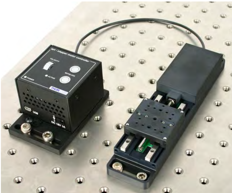
Fig. 2.1 Typical MTS stage and driver set up
